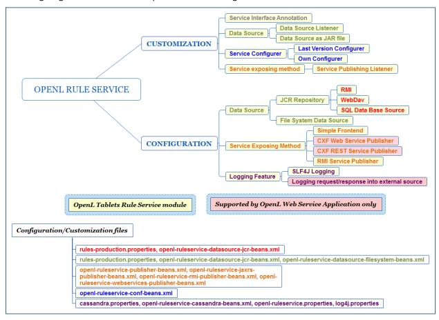
Figure 2: Configurable and customizable components of OpenL Tablets Rule Service
